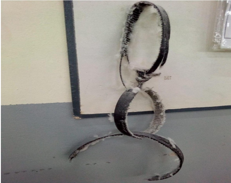
Figure.2.8: Sample of belt that depicts early worn-out failure (REAL maintenance department)
