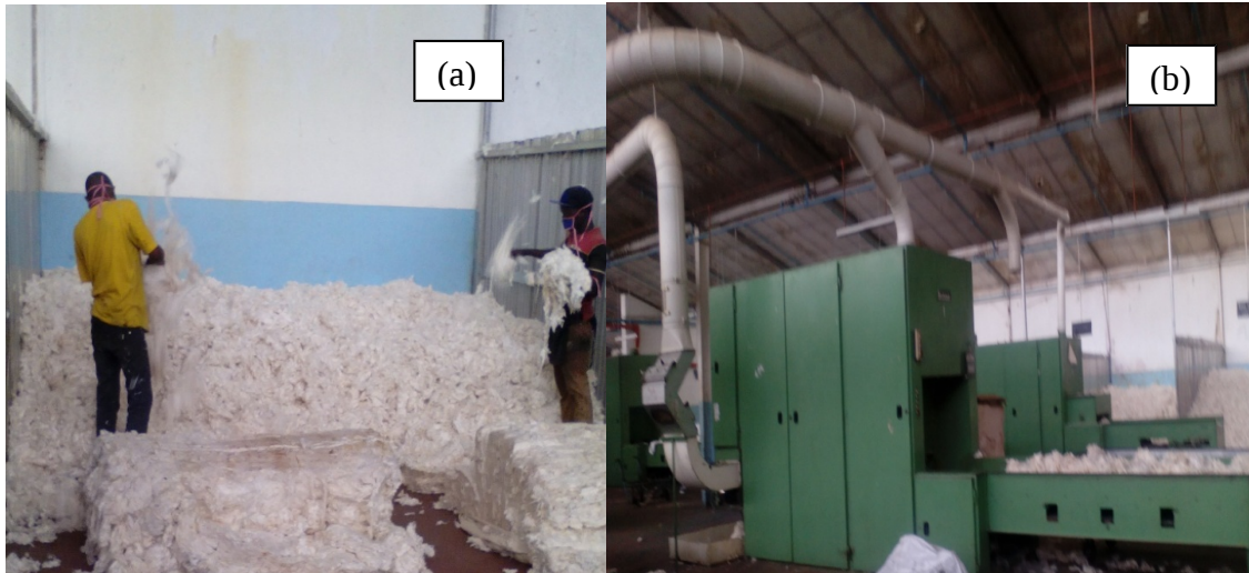
Figure 3.10: (a) Bale opening and mixing and (b) sample on the breaker machine.
