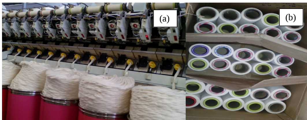
Figure 3.14: Yarn production on a rotor machine and spun yarns in a box.
