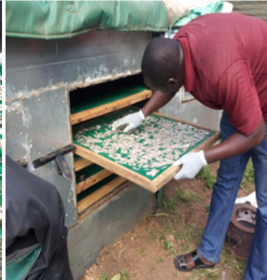
Figure 6. Loading the wet sample into the dryer
