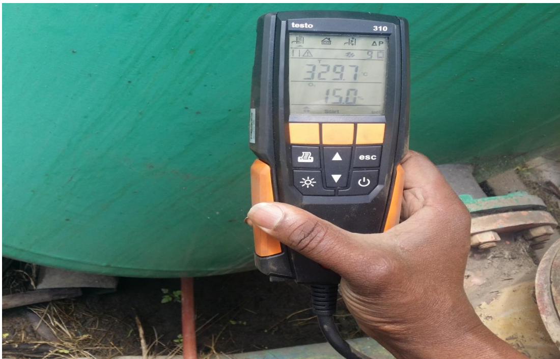
Figure 3.4: A typical display of flue gas temperature and oxygen readings on flue gas analyzer
