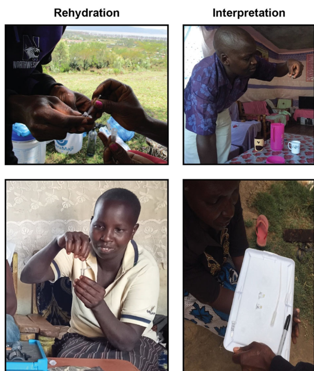
Fig. 3 Representative photographs of experiences with point-of-use fluoride biosensor usability. The two key user activities for operating the tests are test rehydration, in which a micropipette is used to transfer a water sample into a microtubule (left) and result interpretation, in which the user ascertains if a yellow color has appeared (right).
