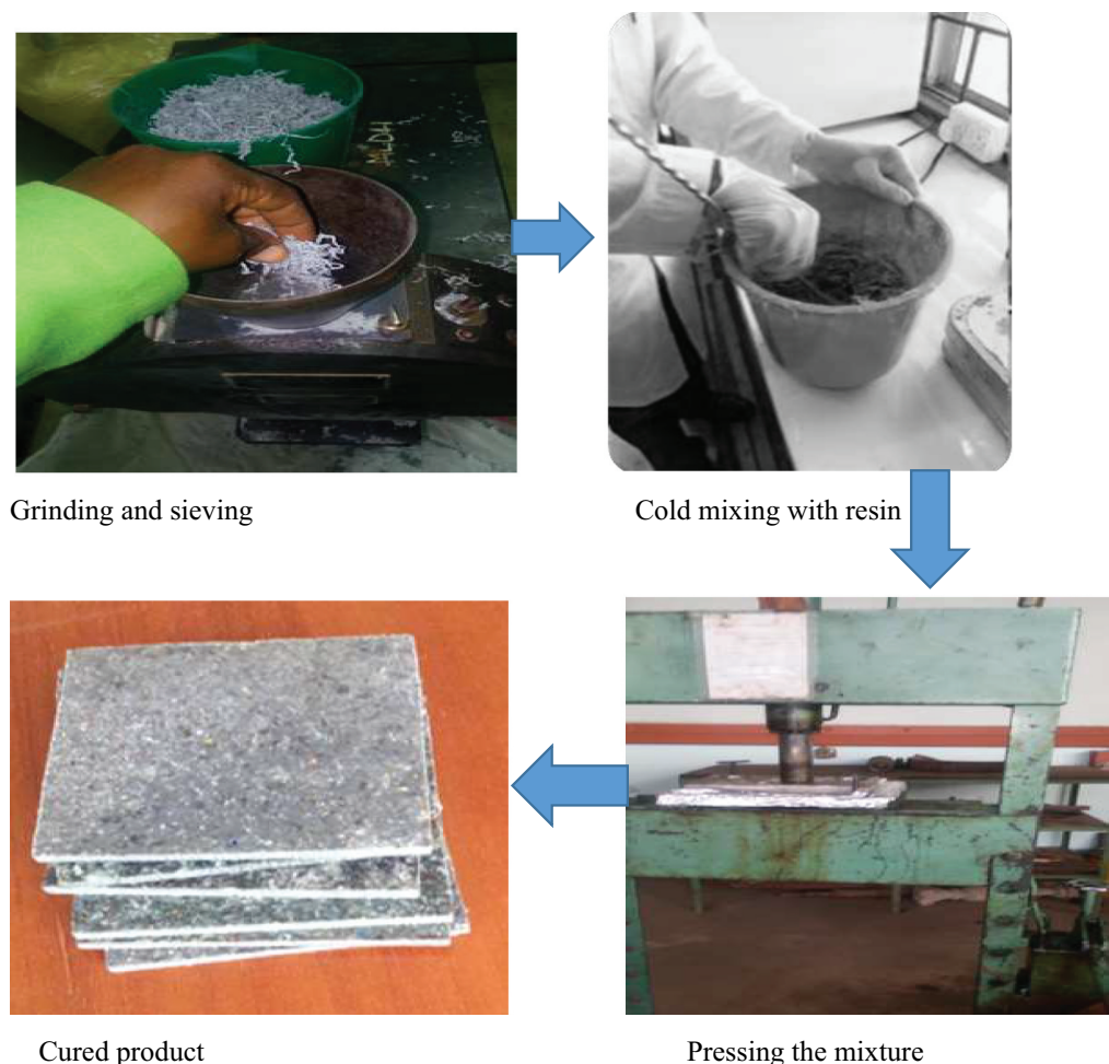
Figure 2. Fabrication process of the particleboard.
