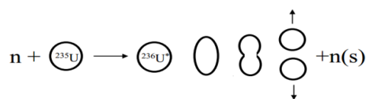
Figure 3. 4: Fission Uranium (U-235) nuclei with a neutron resulting in the formation of two lighter daughter nuclei and neutrons (Cohen et al., 2018).
