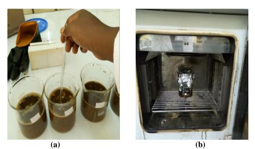
Figure 3.4: (a) Sweet potato waste suspended in NaOH solution and (b) Thermochemical pre-treatment of sweet potato waste
