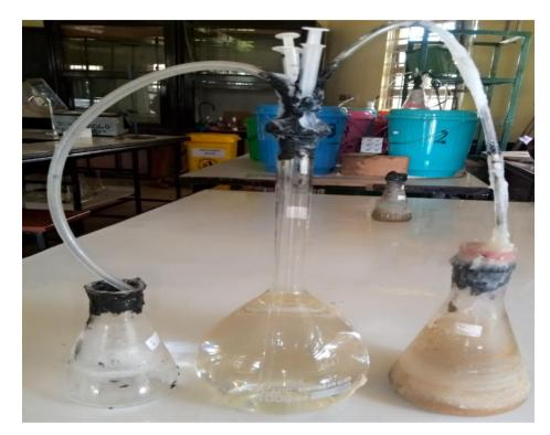
Figure 3.6: Biogas production set up
