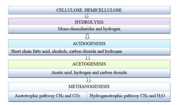
Figure 2.2: Flowchart Sequential steps for AD (Cate et a 2014)
