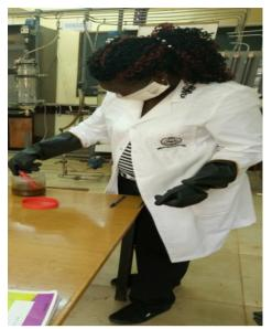
Figure 3.5: Neutralization with HCl and pH testing of pre-treated SPW
