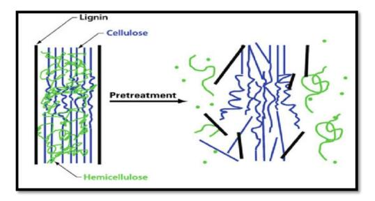
Figure 2.6: Lignocellulosic biomass before and after pre-treatment (Brodeur et al., 2011)
