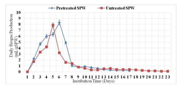
Figure 4 5: Daily biogas productions for the untreated and thermochemically pre-treated SPW for 22 days
