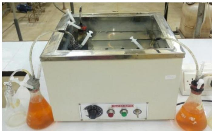
Figure 6.1: Biogas production using varying rumen inoculum percentages
