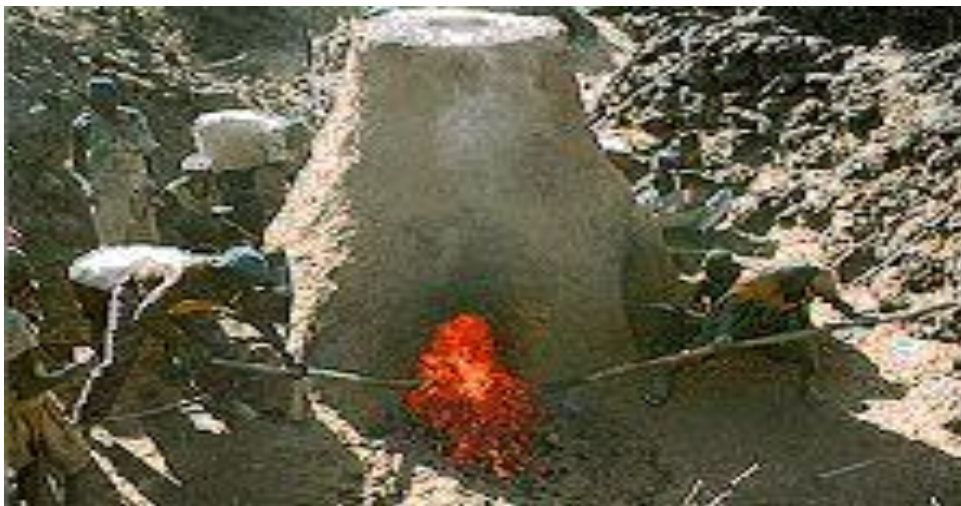
Figure 3.11 A Kiln for Iron Smelting
