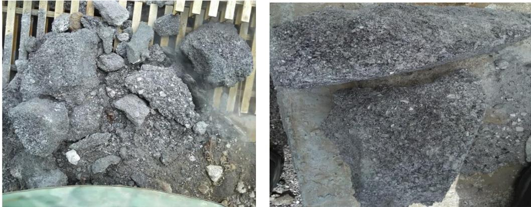
**Figure 4.2:** Images of scale samples collected from the separator –u seal pit
