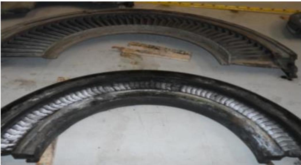
**Figure 2.3:** Turbine blades with silica deposits on nozzles from Olkaria II power plant
