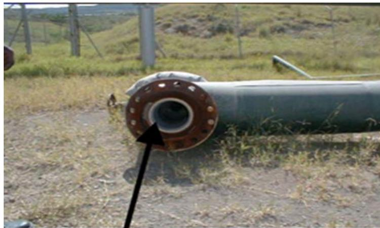
**Figure 4.10:** Thickness of scale at the T-Connection of well 37B
