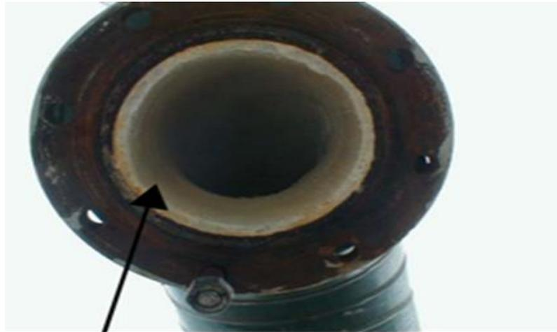
**Figure 4.9:** Thickness of scale deposited in separated water pipeline
