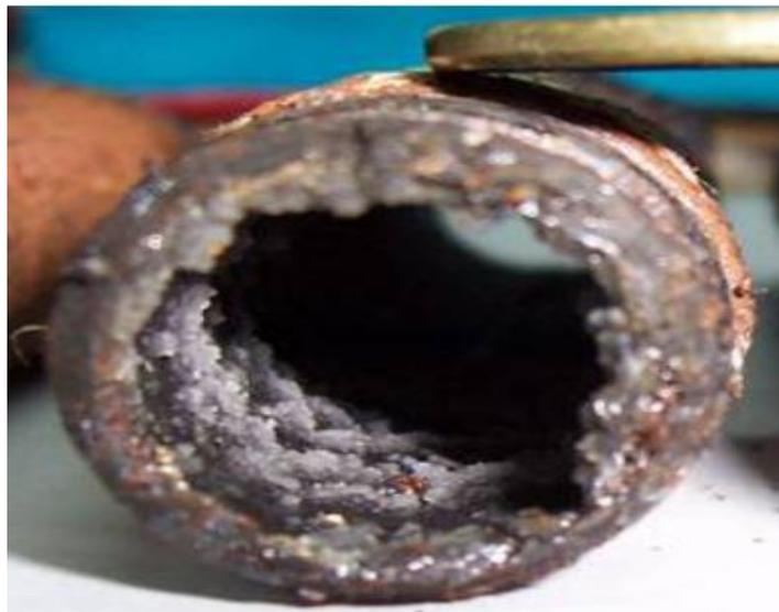
**Figure 1.1:** Shows sample of pipe with thickest silica scale deposit
