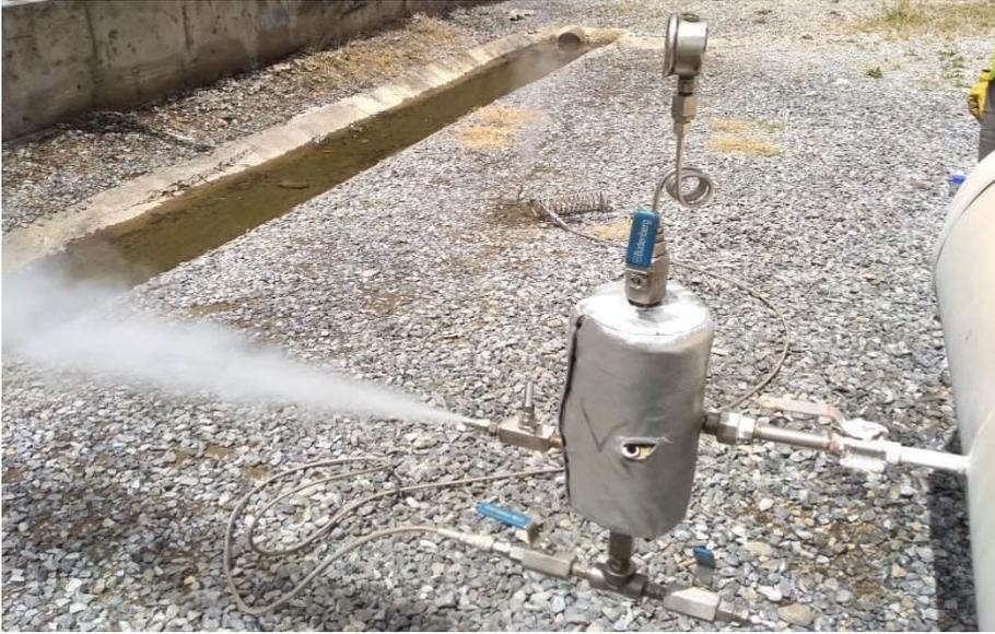
(a) Webre separator connected to a two-phase steam pipe
