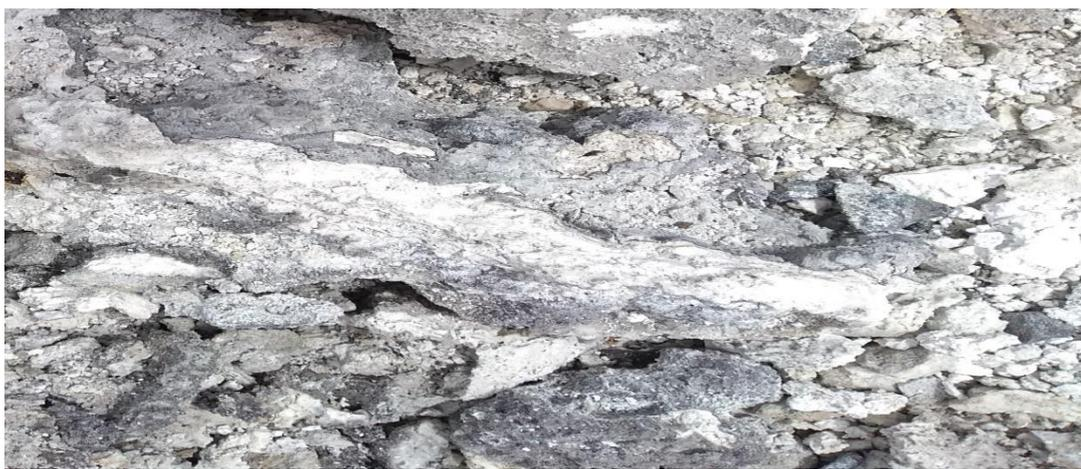
**Figure 4. 6:** An image of scale sample collected from the turbine exhaust
