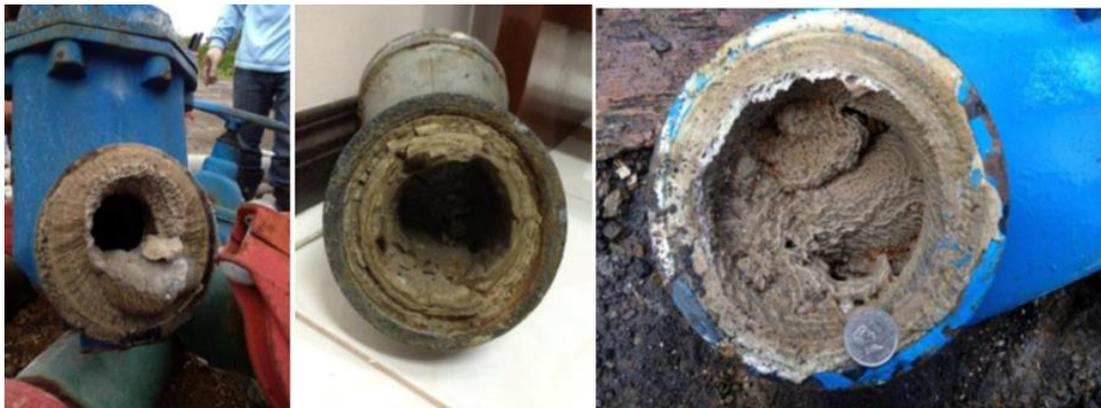
**Figure 1.2:** Massive silica scales depositions at joints, elbows and valves
