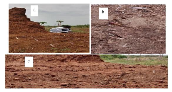
Figure 10: (a): Arrangements of wood blocks around termite nest, (b): Macrotermes natalensis and (c): buried wood block arranged so that the distance between each block is 20 cm and 30 cm from the termite nest.
