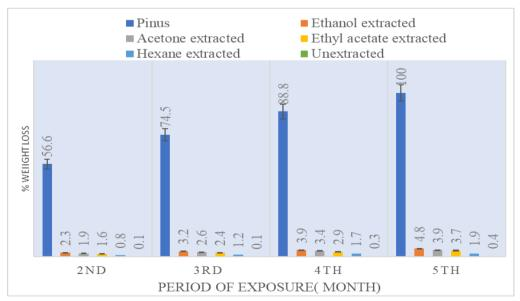
Figure 27: Weight loss of blocks after field exposure for five months
