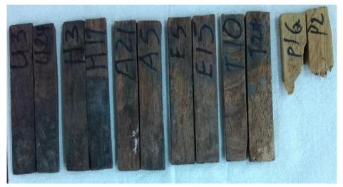
Figure 26: Extent of termite attack on blocks after field exposure for 2 months
