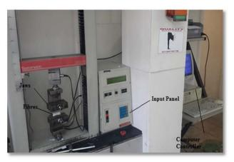
Fig.4Testometric micro 500 used for fibre tenacity testing
