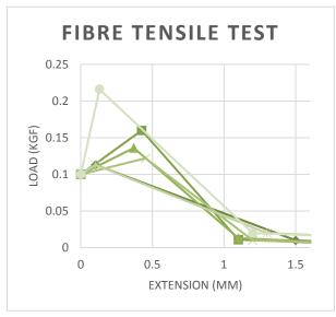
Fig 8–Load/extension curve for Cotton stalk fibres fromtop section
