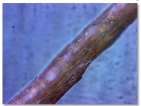
Fig 13 Microscopic image of cotton stalk fibre 4X magnification
