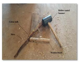
Fig. 2 Fibre extraction
