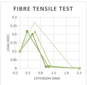
Fig 7– Load/Extension curve for cotton stalk fibres from bottom section
