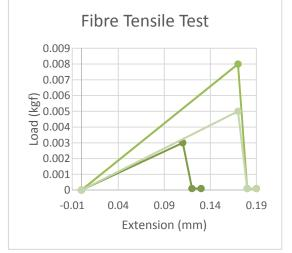
Fig 9– Load/extension curve for Cotton stalk fibres from root section
