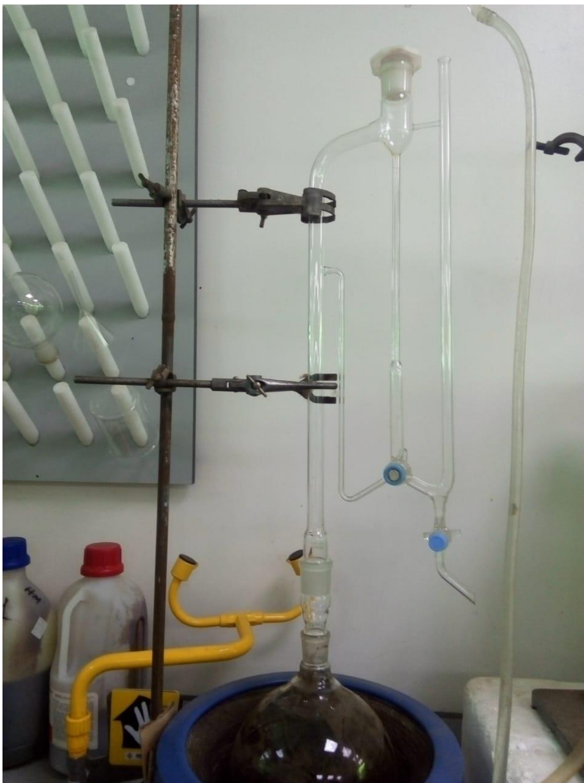
Fig. 8: Soxhlet extraction for essential oils. Photo by the authors.
