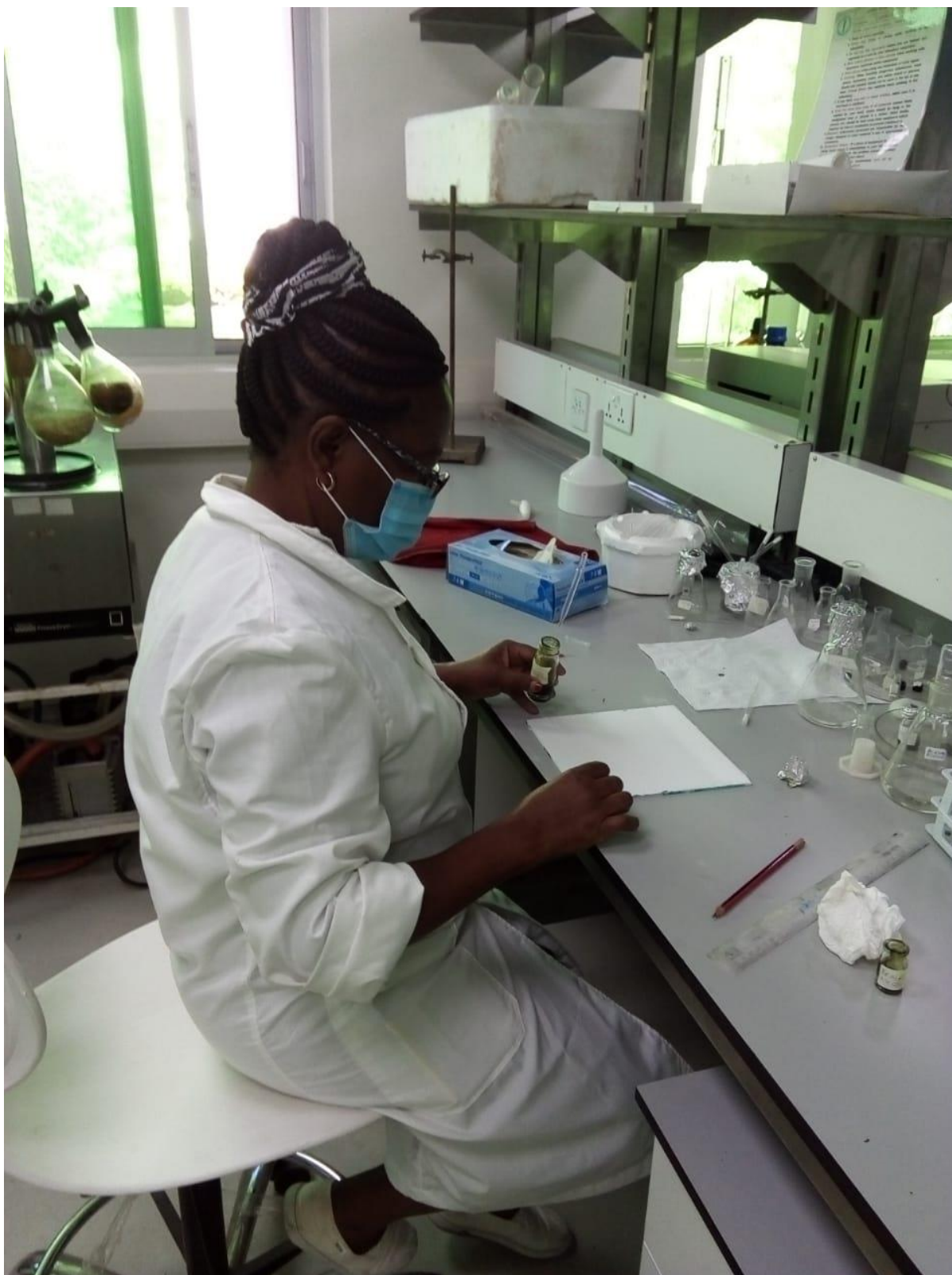
Fig. 14: Dr. Dorcas Lusweti spotting the algal extracts on a TLC plate. Photo by authors.
