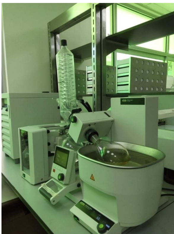
Fig. 3: Drying of the extracts on a rato-vaporator (Rotavopor R-300). Photo by author.
