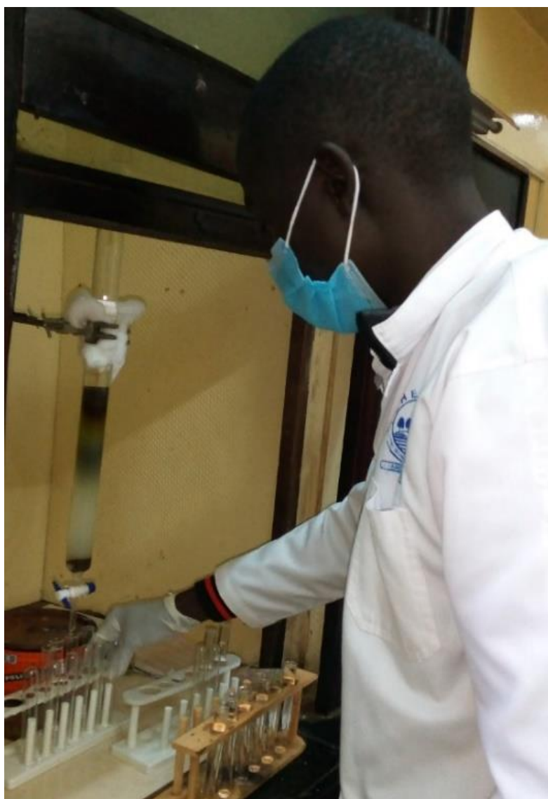
Chromatographic isolation of compounds in ethanolic extracts of A. coriaria leaves from Mbarara using hexane: ethyl acetate (9:1) solvent system.
