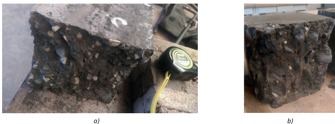
Fig. 4. Failure pattern of specimens: a) Beam Failure under Flexural Test, b) Cube Failure under compressive strength test.
