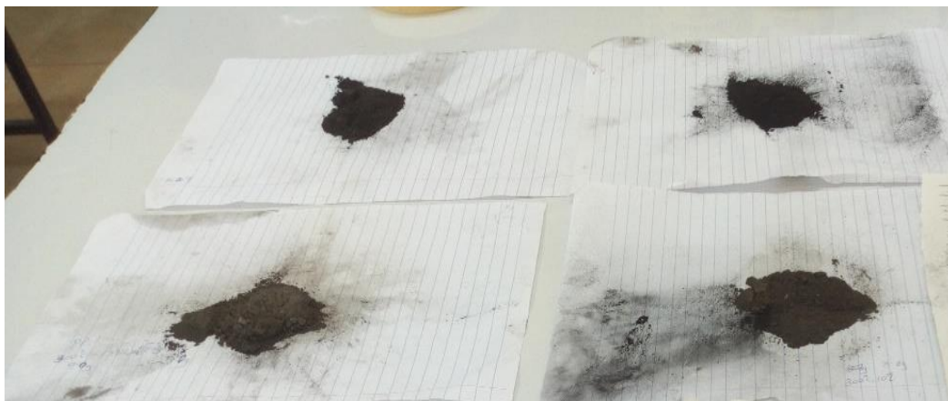
Appendix 1f: Char (By product of pyrolysis process)
