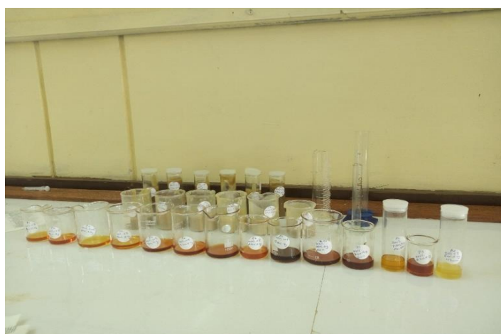
Appendix 1e: Pyrolytic oil for HDPE, PP and PS
