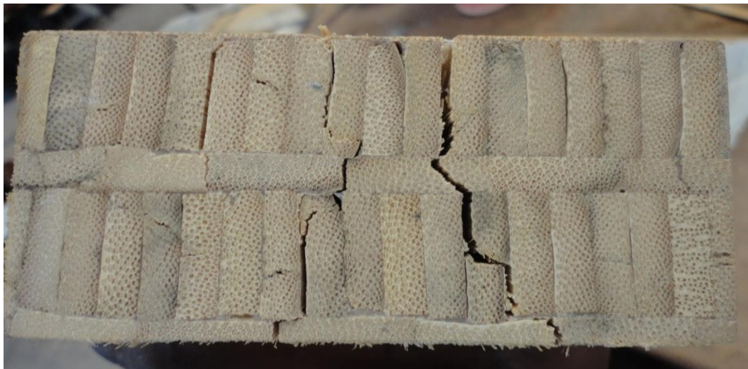
Figure 8 Failure pattern at the edge of bamboo laminated beam
