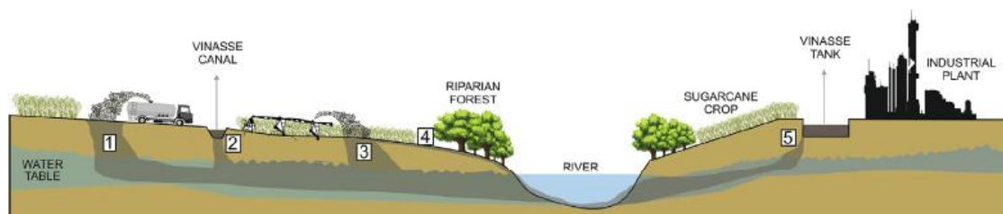
Figure 2.9: Main forms of introduction of Vinasse into water bodies: (1) and (3) Percolation from fertirrigation; (2) Percolation from a vinasse canal spill; (4) Runoff over soil; (5) Percolation from a vinasse tank. (Carrilho et al. , 2017)
