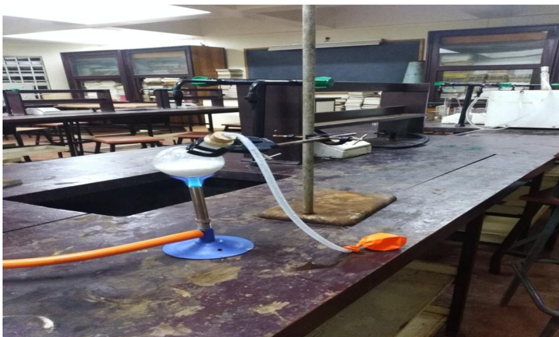
Figure6.4: Standard methane gas preparation experiment setup
