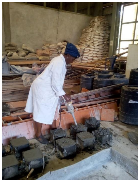
Compacting the mixture
