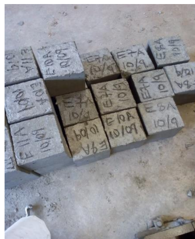
Cubes ready for curing
