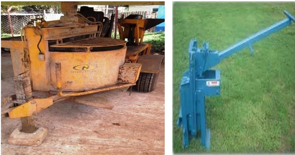
**Figure 4.4 the motorized versus the manual block press machine**
