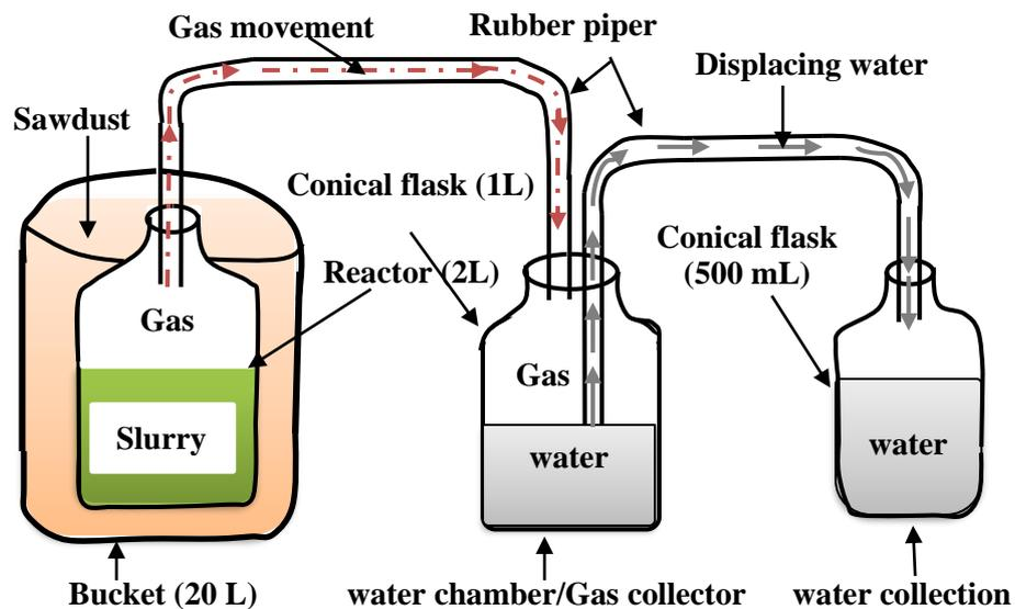
**Figure 3.13: Overview for model biogas plant**
