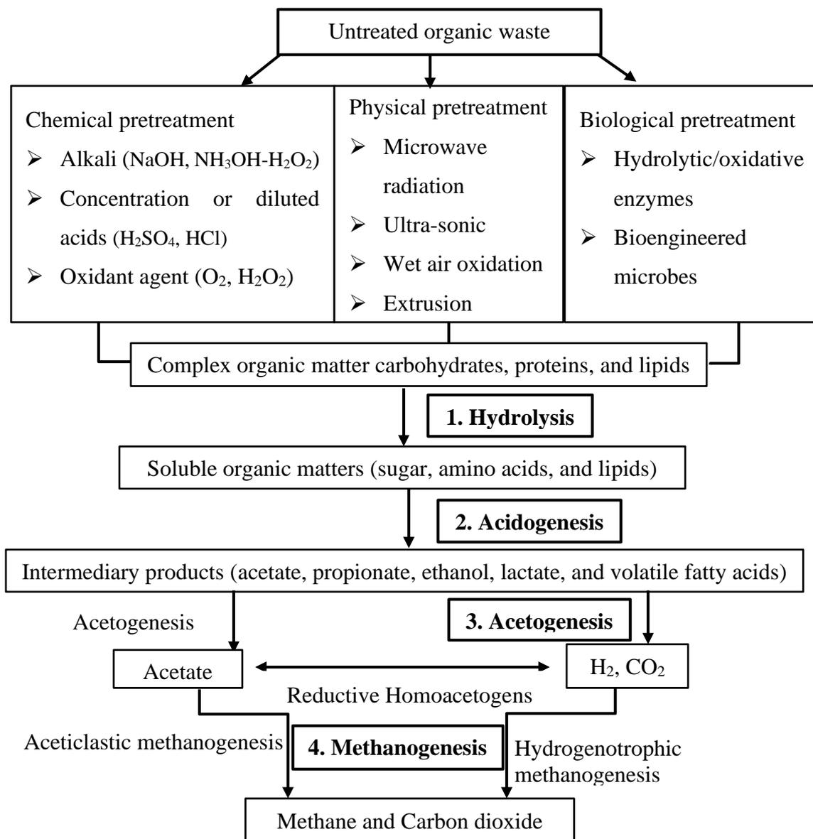
**Figure 2. 1: Pre-treatment methods classification and AD process for biogas production** modified from (Andriani et al., 2014; Mir et al., 2016a)
