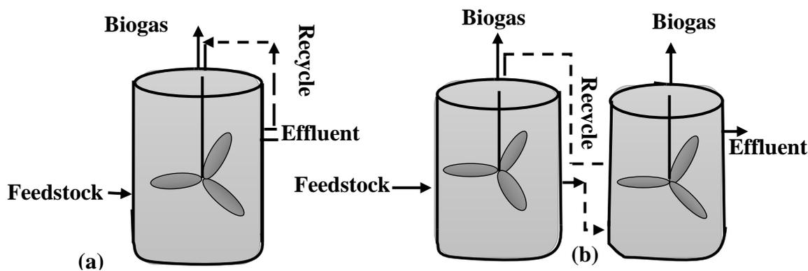
**Figure 2. 5: Design variations in (a) one-stage and (b) two-stage reactors (Nizami & Murphy, 2010).**
