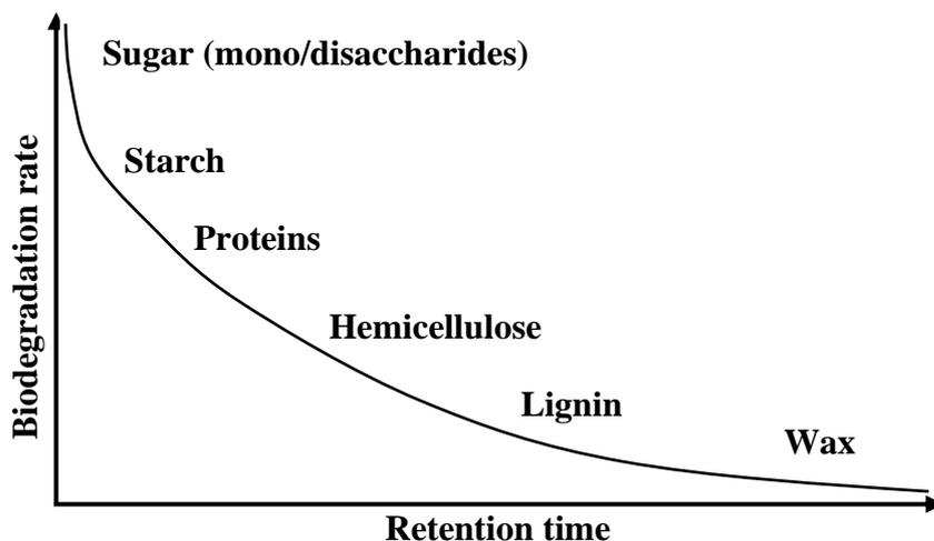
**Figure 2. 4: Relationship between the speed of degradation and retention time reckoning on the type of organic compound (AKUNNA, 2018)**
