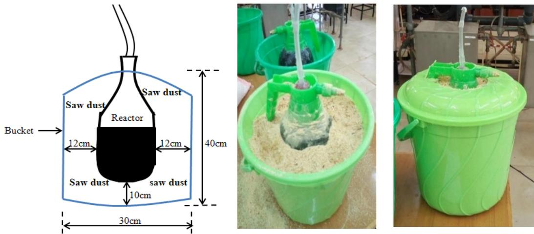
**Figure 3.12: Reactor buried in a bucket filled with sawdust**
