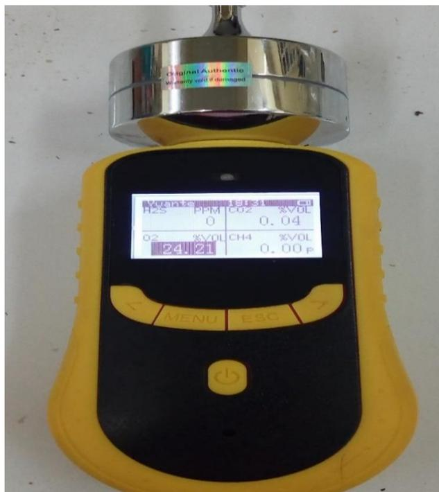
**Figure 3. 4: A multi-gas detector used in the analysis of biogas yield**
