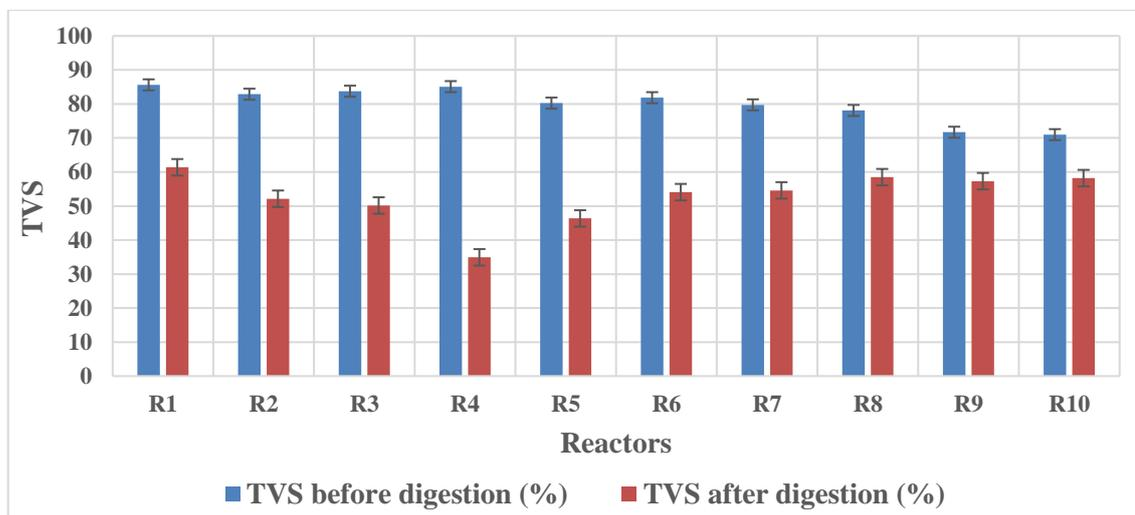
**Figure 4. 5: Content variation of TVS before and after the anaerobic digestion**
