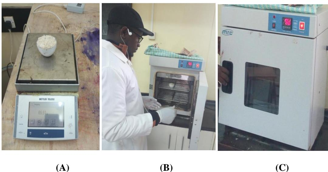
**Figure 3. 9: (A), (B), and (C) show the determination of the weight of the crucible with material by using analytical balance before putting the samples into the oven and after setting the oven at 105 °C.**
