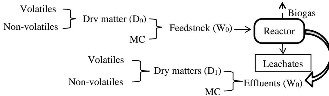
**Figure 3. 11: Materials balance analysis in the anaerobic digestion process**
