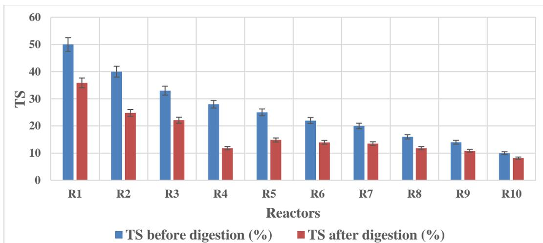
**Figure 4. 4: Content variation of TS before and after anaerobic digestion**
