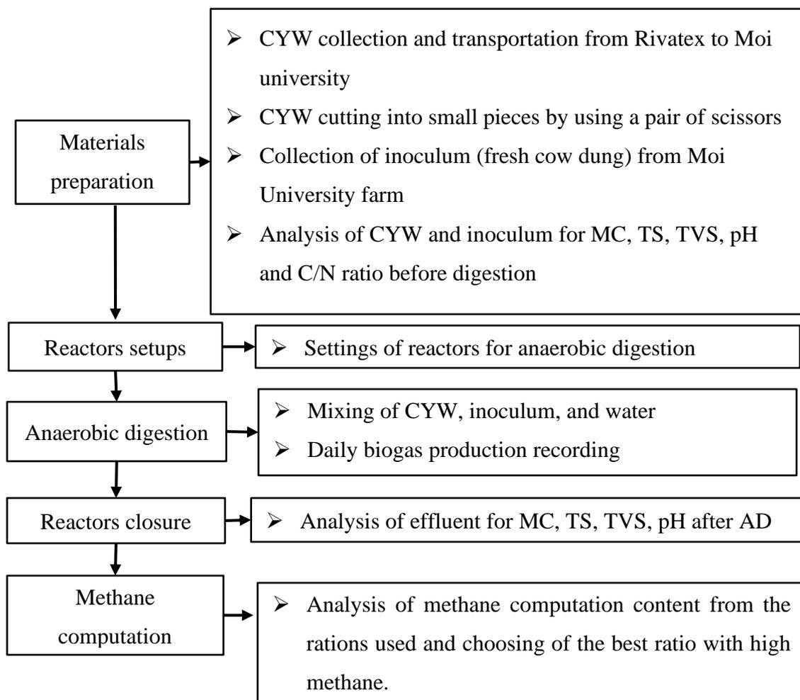
**Figure 3. 1: Process flow diagram**
