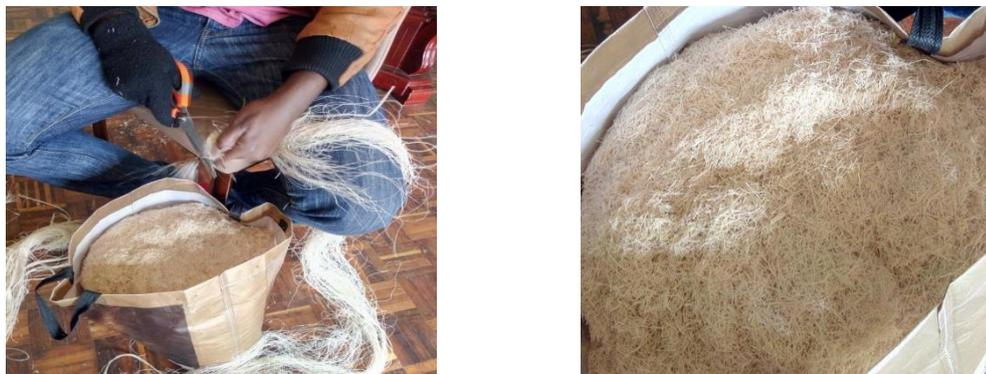
**Figure 3. 7: Cotton yarn wastes bulk sample after cutting into small pieces.**
