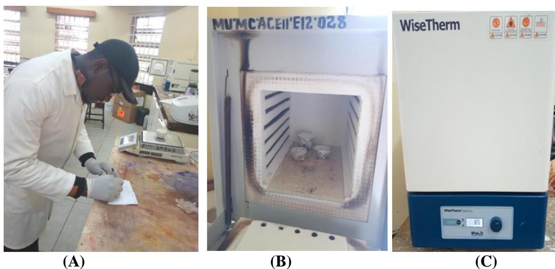
**Figure 3. 10: (A), (B), and (C) show data recording, the dry matter within the furnace and furnace settled at 550 °C.**
