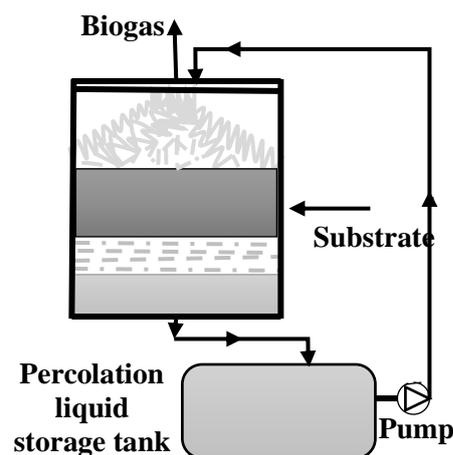
**Figure 2. 6: One-stage dry batch reactor with a sprinkling of liquor in a very controlled system (Nizami & Murphy, 2010)**
