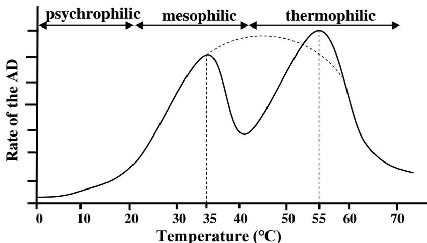
**Figure 2. 7: Rate of AD process vs temperature** (Velmurugan et al., 2014)
