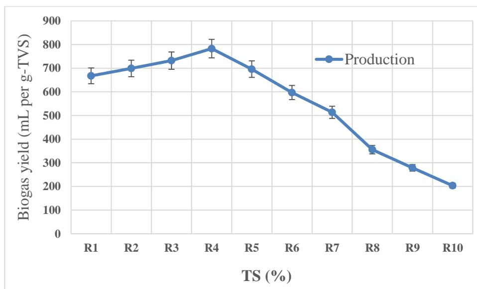
**Figure 4. 3: Effect of TS on biogas yields. R1 to R10 represent 50, 40, 33, 28, 25, 22, 20, 16, 14 and 10% respectively**
