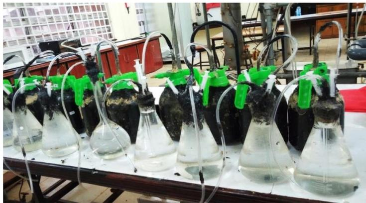
**Figure 3.14: The prepared reactors filled with slurry and water displacement**
