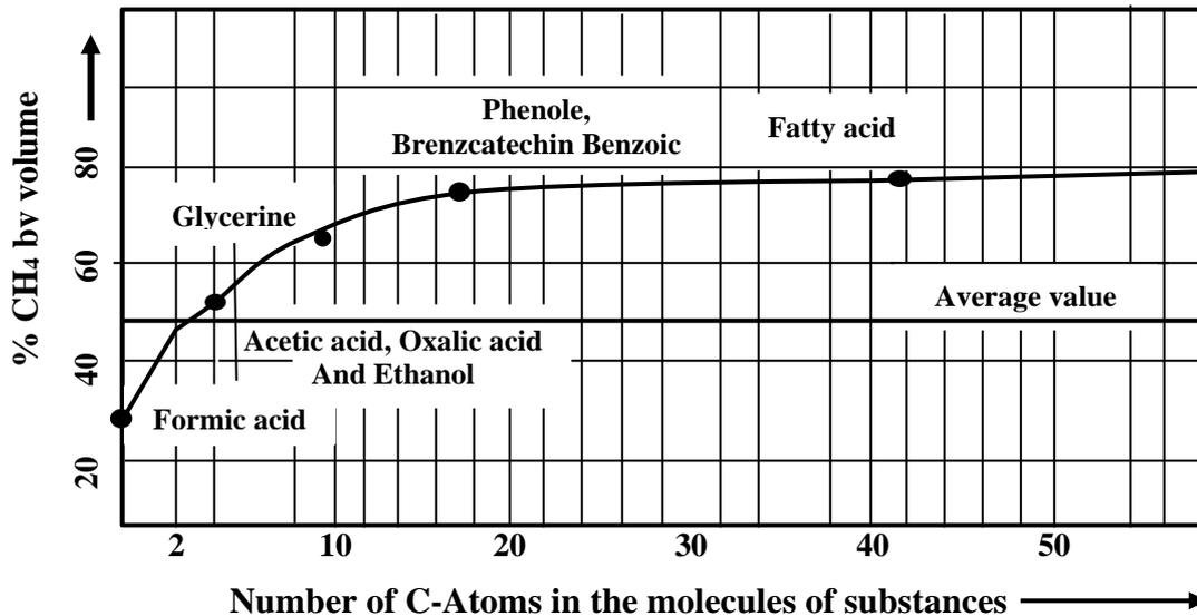
**Figure 2. 2: A statistical relation between CH<sub>4</sub> content in biogas and the number of carbon atoms (Rajendran et al., 2011)**
