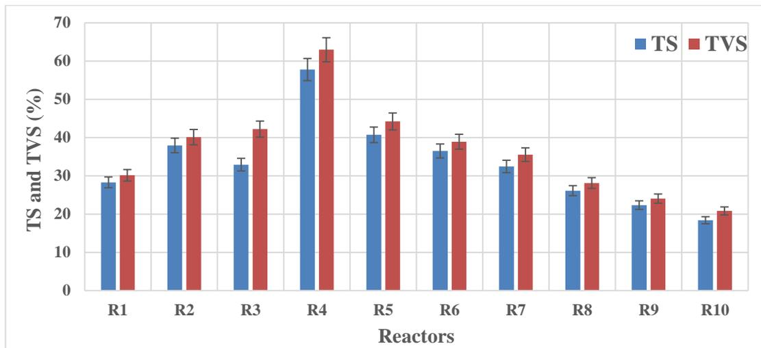
**Figure 4. 6: The TS and TVS reduction after digestion**
