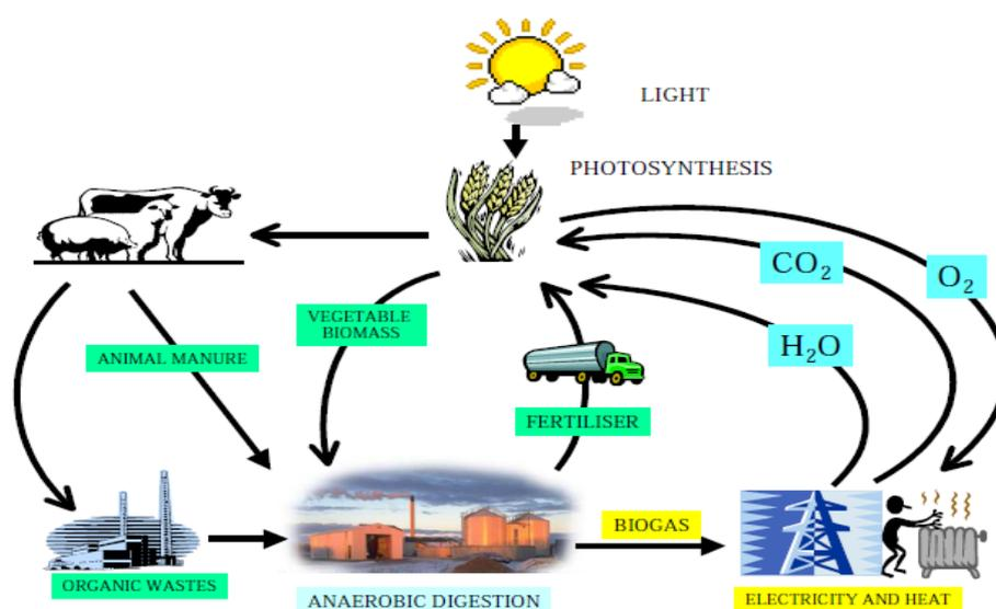
**Figure 2. 3: The sustainable cycle of biogas from AD (Seadi et al., 2008)**
