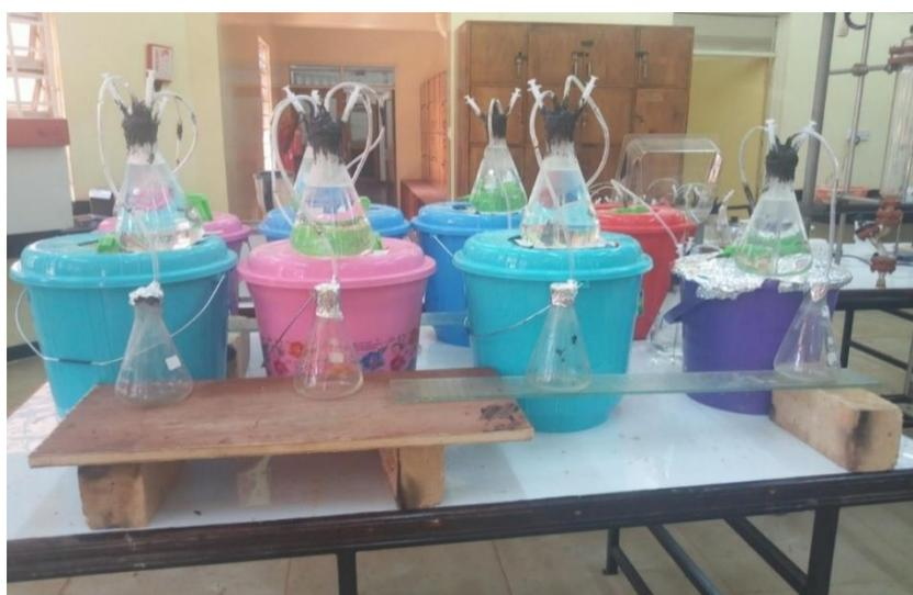
**Figure 3.15: Full biogas set up**
