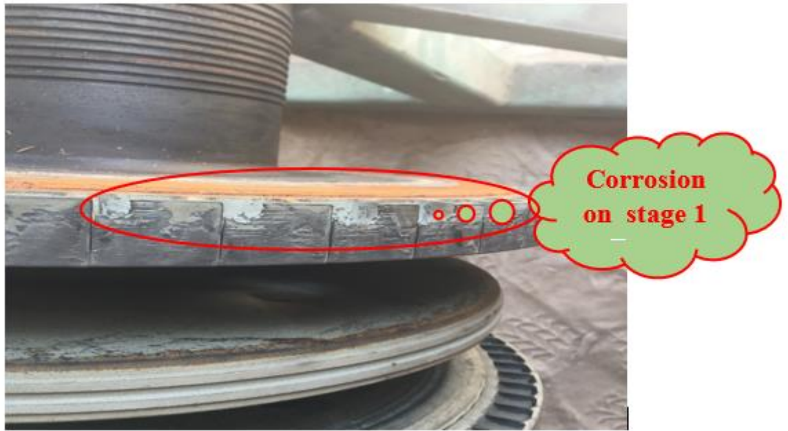
Plate 1.1: Corrosion on stage 1 Rotor blade
