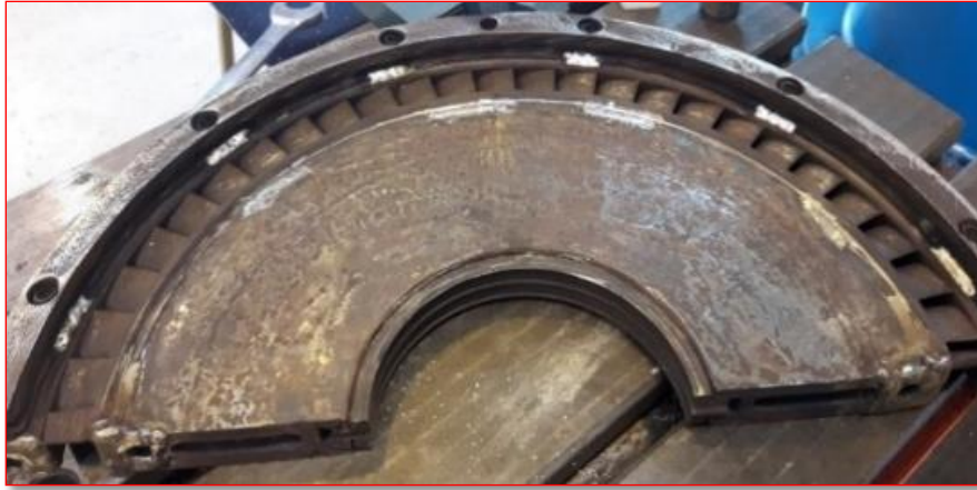
Figure 3. 7: Weld repaired diaphragm (Source: Researcher, 2019)
