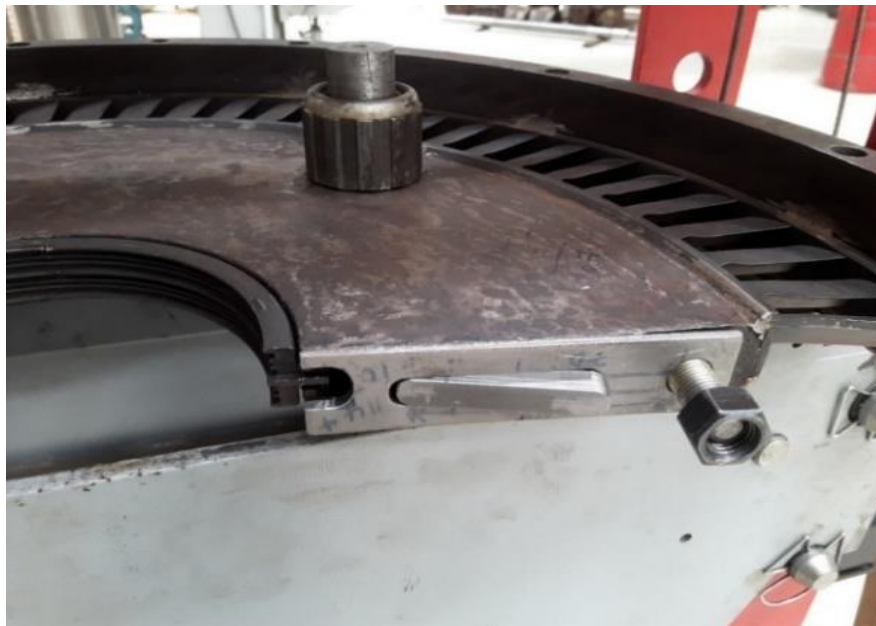
Figure 3. 10: Repaired diaphragm fitted with key lock and assembling bolt & nut (Source: Researcher, 2019)
