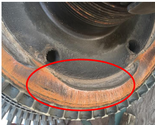
Plate 1. 2: corrosion on rotor
