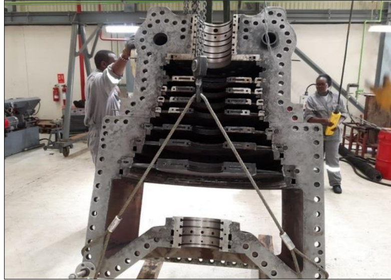
Figure 3. 13: Assembled Upper Casing after repairs (Source: Researcher, 2019)
