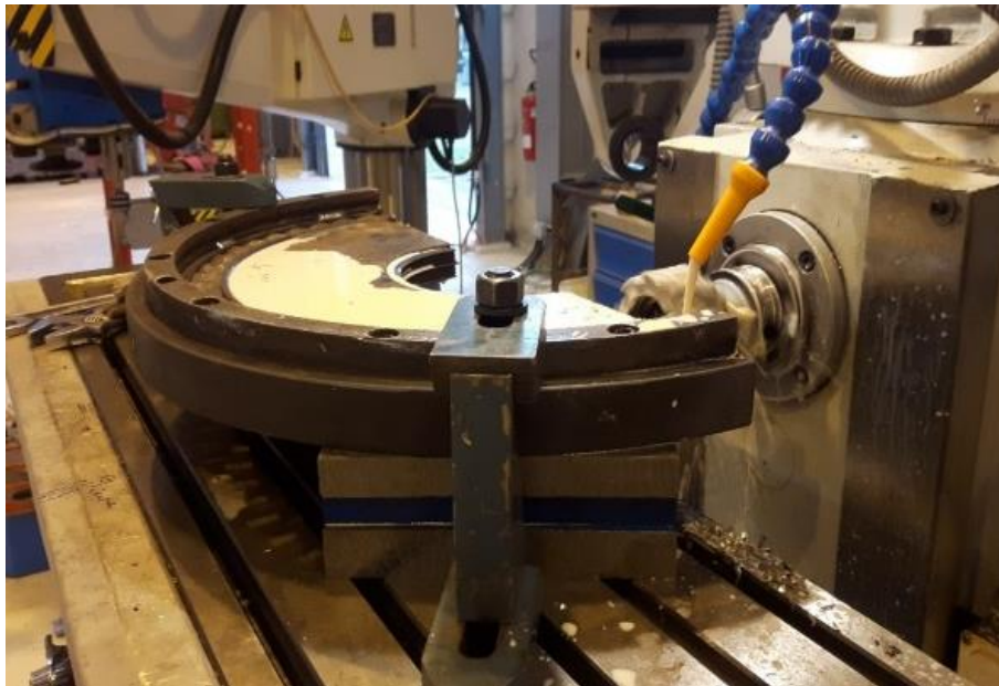
Figure 3. 8: Milling of repaired diaphragm split line face (Source: Researcher, 2019)
