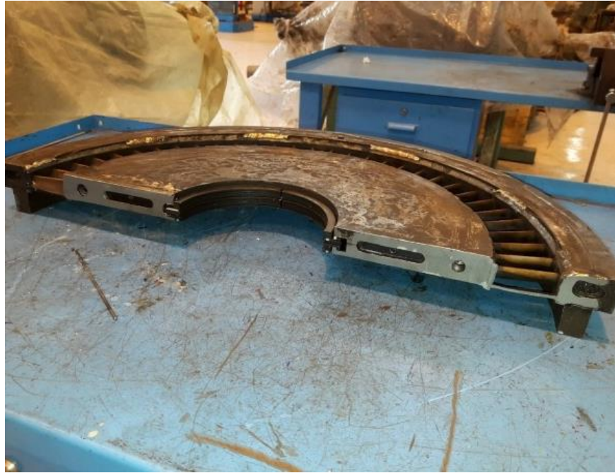
Figure 3. 9: Repaired Diaphragm (Source: Researcher, 2019)
