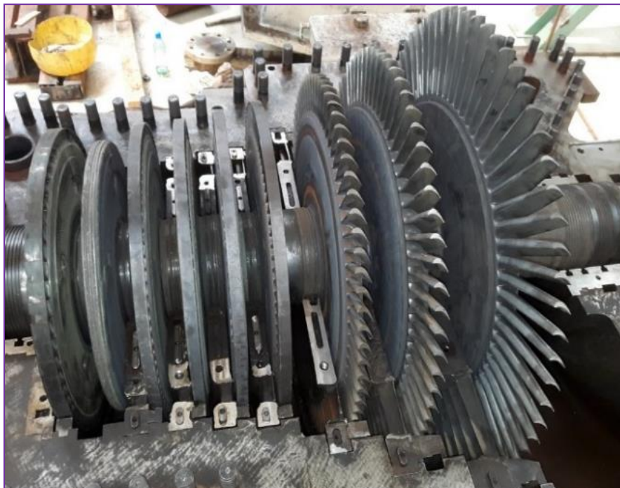
Figure 3. 12: Reassembled rotor after repairs (Source: Researcher, 2019)
