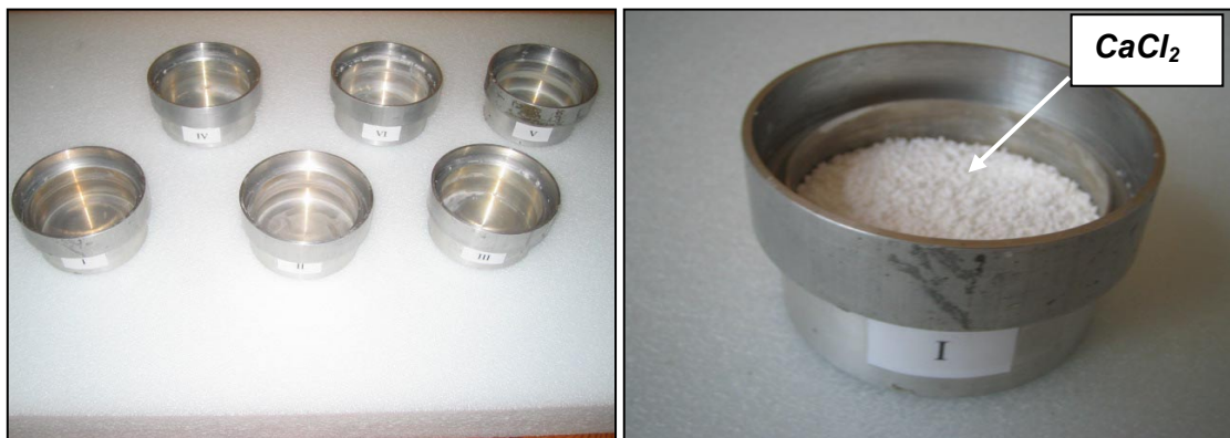
Figure 6.47 Empty cup and one containing vapour pressure regulator
