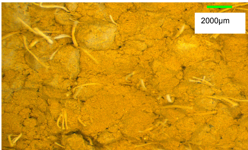
Figure 6.14 Fractured surface of a 1.0% sisal reinforced block
