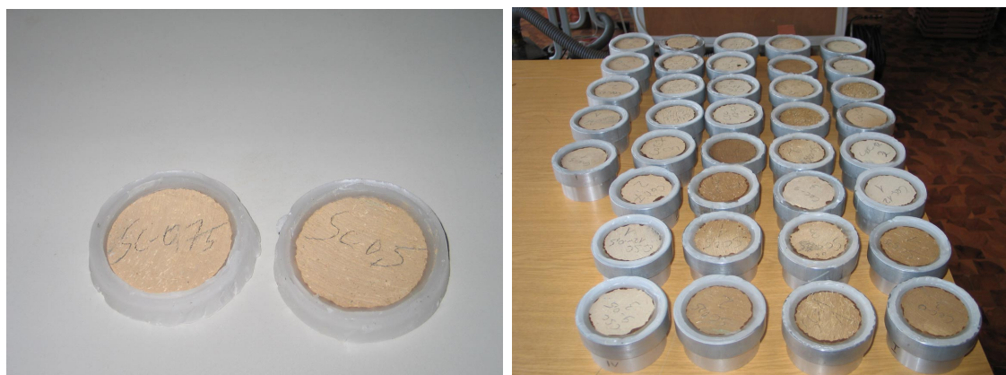
Figure 6.48 Prepared samples (left) and cups with sealed test specimen
