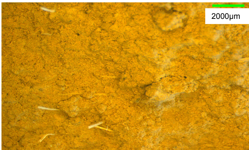
Figure 6.11 Fractured surface of a 0.25% sisal reinforced block
