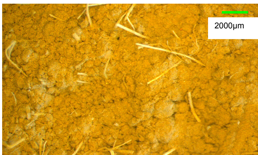
Figure 6.12 Fractured surface of a 0.5% sisal reinforced block
