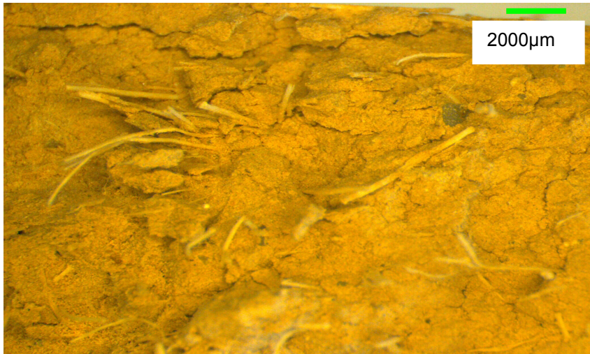
Figure 6.13 Fractured surface of a 0.75% sisal reinforced block
