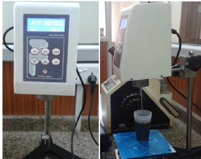
FIG. 1. Rotational Viscometer for bio-resin characterization.
