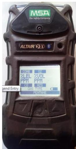
**Plate 3.8: Digital Gas Analyzer**
