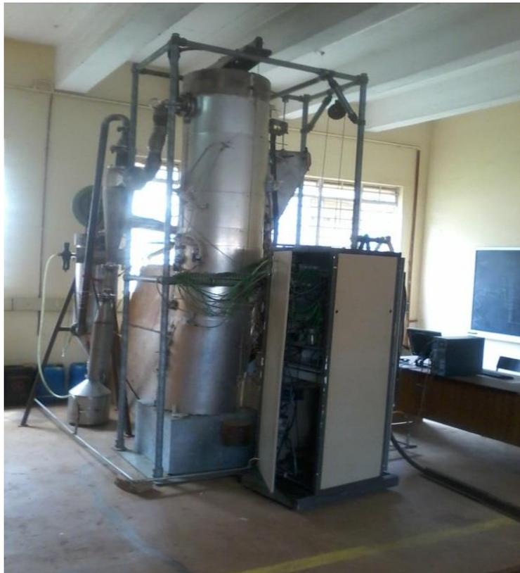
*Plate 3.1: Fluidized bed combustor Moi University FL laboratory*
