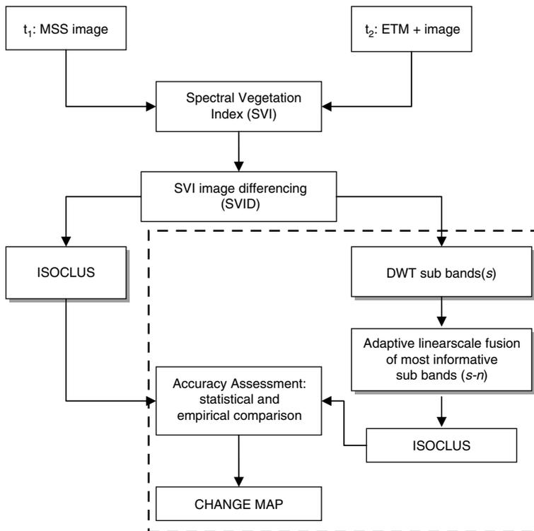
Figure 3. Block scheme of the proposed change-detection approach.  $t_1$  and  $t_2$  are the two time epochs corresponding to MSS and ETM+, respectively, and DWT is the discrete wavelet transform. (The dotted outline is the DWT–ISOCLUS algorithm).
