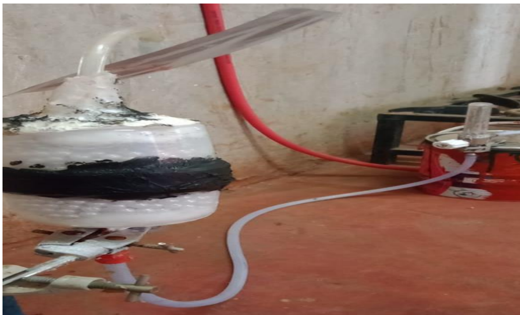
Plate 3.7: - The set-up of biogas upgrade using dry adsorbent
