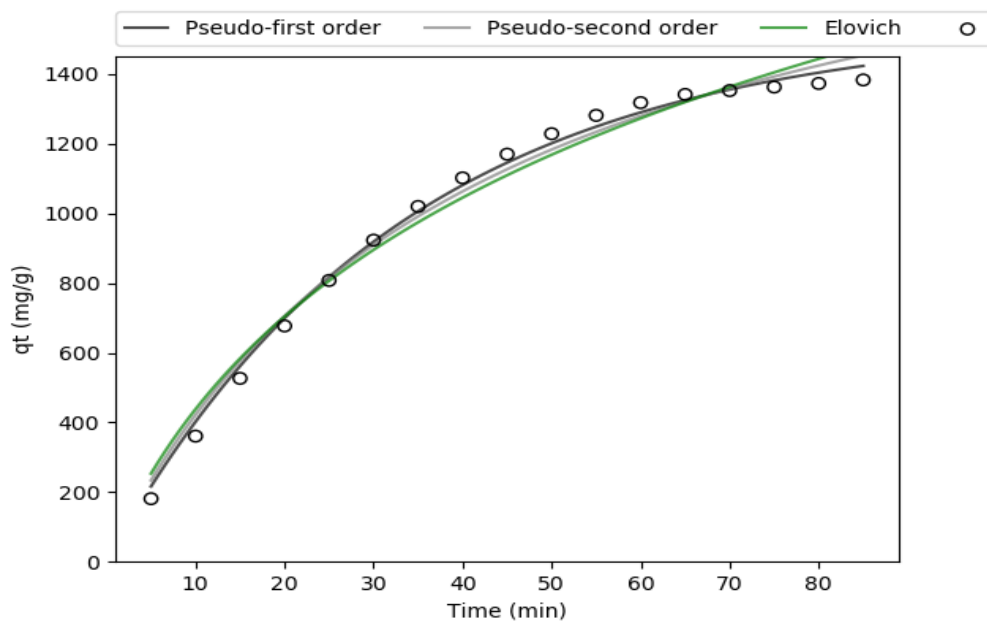
Figure 4.10:- Kinetic plot of carbon dioxide uptake using activated clay for pseudo-first order, pseudo-second order, elovich and intra particle diffusion models
