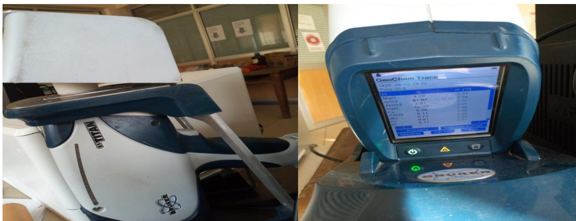
Plate 3.5:- Characterization of the chemical components of adsorbent using X-ray fluorescence
