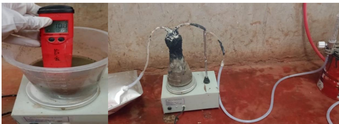
Plate 3.6:- The setup of biogas upgrading by carbonation process
