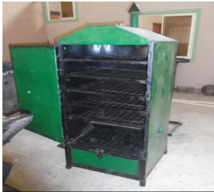
Figure 2.15: A Simple hybrid maize dryer (Adekanye., 2016)
