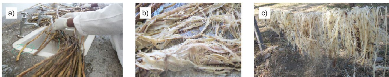
Figure 2. Extraction of Kenyan hibiscus fibres; a) extracting the fibres from retted stem, b) extracted bast fibres, c) drying of the extracted bast fibres.
