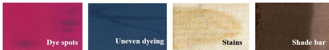
Figure 1.1: Defects in dyed fabrics (taken from local textile industries in Kenya)
