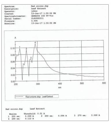
Fig. 7: Absorption spectrum for red onion extract
