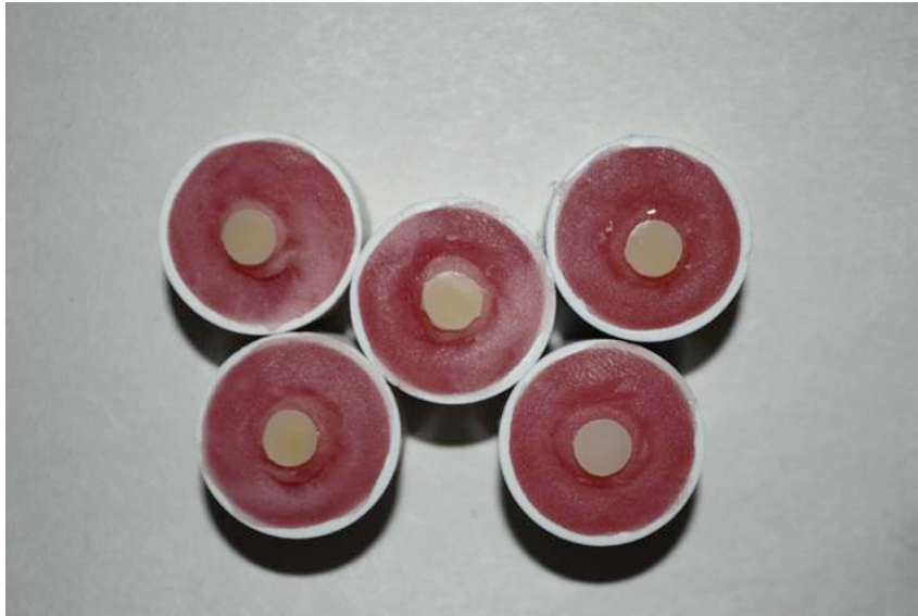
Figure 15: 5mm X 5mm composite cylinders after embedding in acrylic resin
