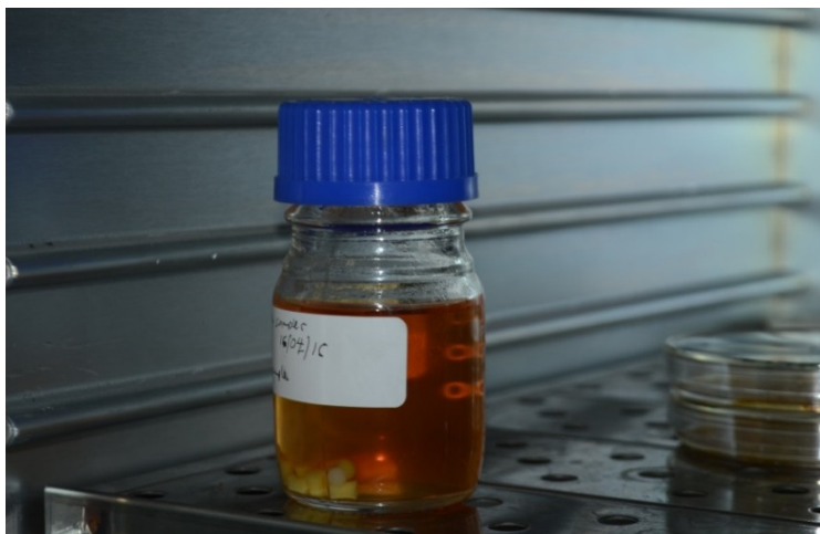
Figure 14: Composites cylinders undergoing aging in artificial saliva within an incubator
