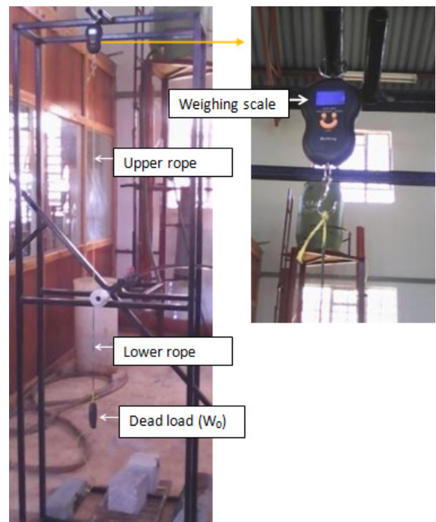
Figure 3. Rope Brake dynamometer with a digital weighing machine
