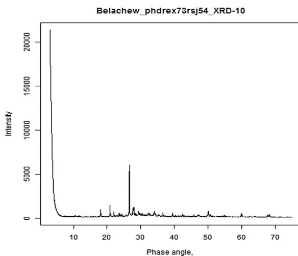
From Table 15 and diagrams Figures 6–9, it can be shown that the main mineral phases of RRPC containing fly ash and glass powder are Albite ( $\text{NaAlSi}_3\text{O}_8$ ), Calcite ( $\text{CaCO}_3$ ), Microcline ( $\text{KAlSi}_3\text{O}_8$ ), Portlandite ( $\text{Ca}(\text{OH})_2$ ) and Quartz ( $\text{SiO}_2$ ). Accordingly, the mineralogical composition for main mineral
