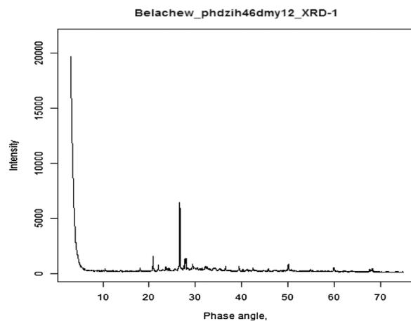
Figure 7. XRD pattern of RRPC mix containing 50FA–50GP.
