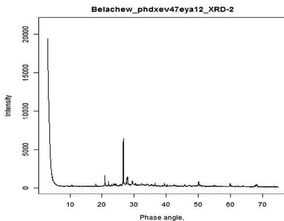
Figure 8. XRD pattern of RRPC mix containing 75FA–25GP.
