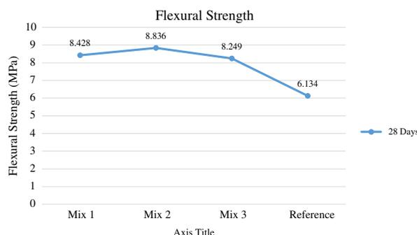
is defined as a property of a material or structural member that indicates its ability to resist failure in bending. Figure 5 shows the flexural strength of RRPC beams with different percentages of fly ash and finely dispersed glass powder. Accordingly, a maximum flexural strength 8.8 MPa was observed using Mix 2. Compared to the reference, 30.58% was improved using the series.
