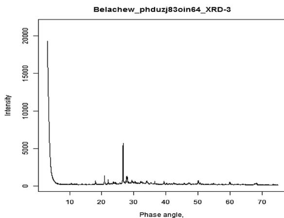
Figure 9. XRD pattern of RRPC mix containing silica fume (ref.).
