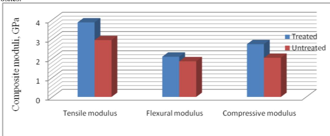
**Figure 2:** Effect of alkali treatment on the tensile, flexural and compressive moduli of the composites
