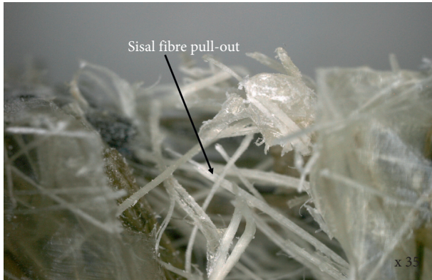
FIGURE 8: Micrograph showing the reinforcing effect of sisal and cattail fibres.
