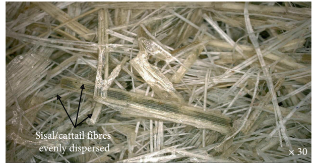
FIGURE 3: Micrograph of the sisal/cattail composite with 20% hybrid fibre weight fraction at constant fibre blend ratio.
