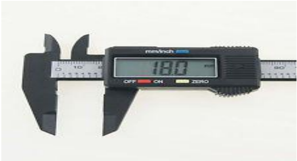
Figure 1: Showing digital Vernier calipers that that was used to measure the linear measurements of the cervical pedicle
