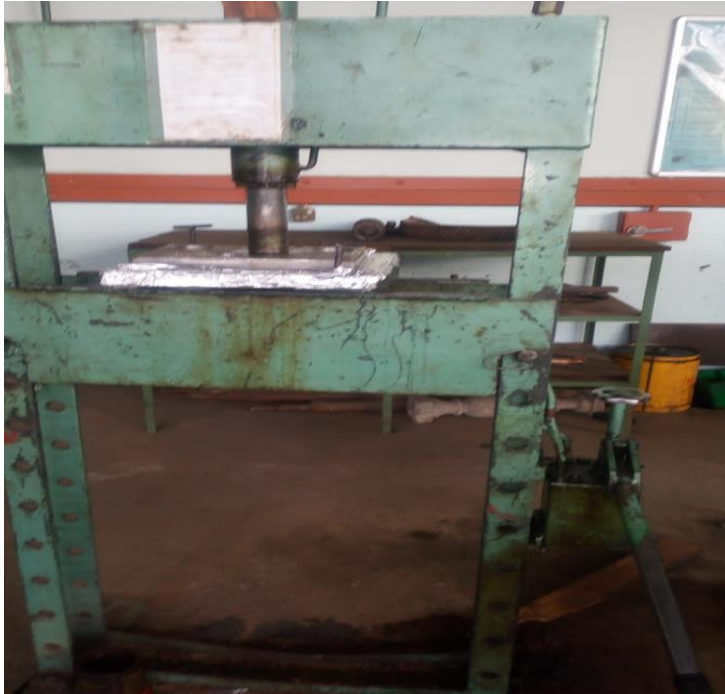
Figure 3.4: Compression of particle board on hydraulic press machine
