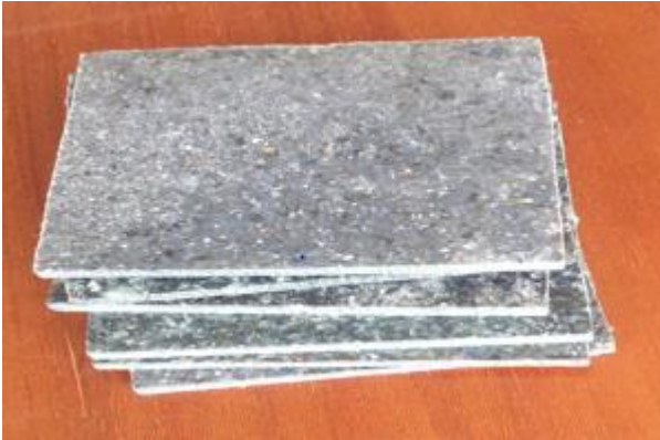
Figure 4.1: Samples of fabricated particleboard
