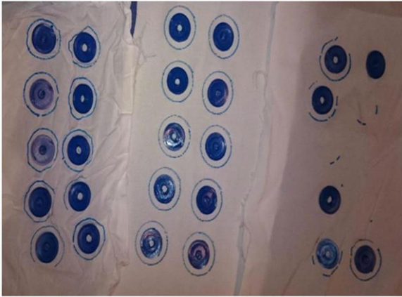
Figure 2.30 : ABS Objects Printed on Different Textile Fabrics after 4 Washing Cycles (Martens & Ehrmann, 2017).
