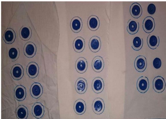
Figure 2.29 : ABS Objects Printed on Different Textile Fabrics after 1 Washing Cycle (Martens & Ehrmann, 2017).
