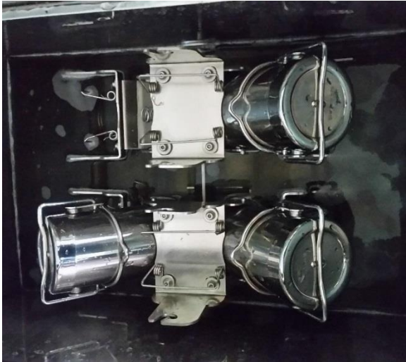
Fig. 3.10 : Setting of the Steel Containers in the M228 Rotawash.
