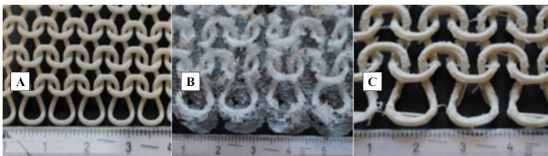
Figure 2.14 : Single-Faced Weft Knitted Fabric printed with (A) SLS and Nylon, (B) FDM and Bendlay , (C) FDM and Soft PLA (Melnikova, Ehrmann, & Finsterbusch, 2014).
