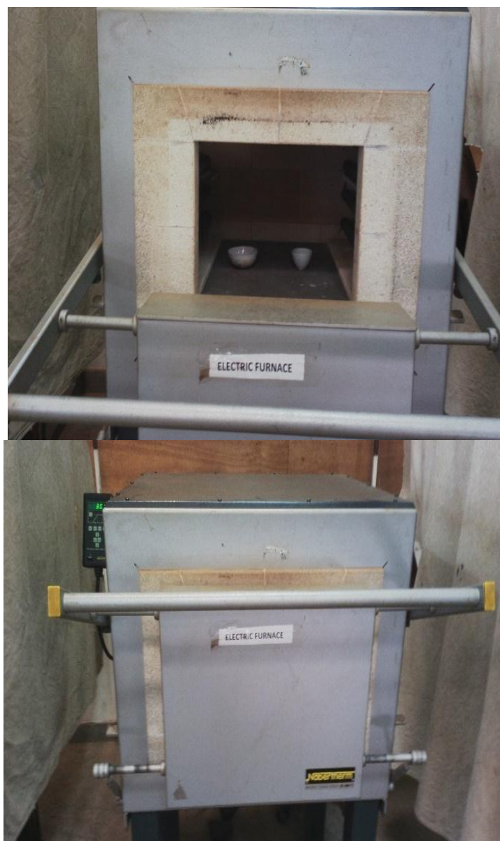
Figure B.2: Furnace used to calcine the catalyst
