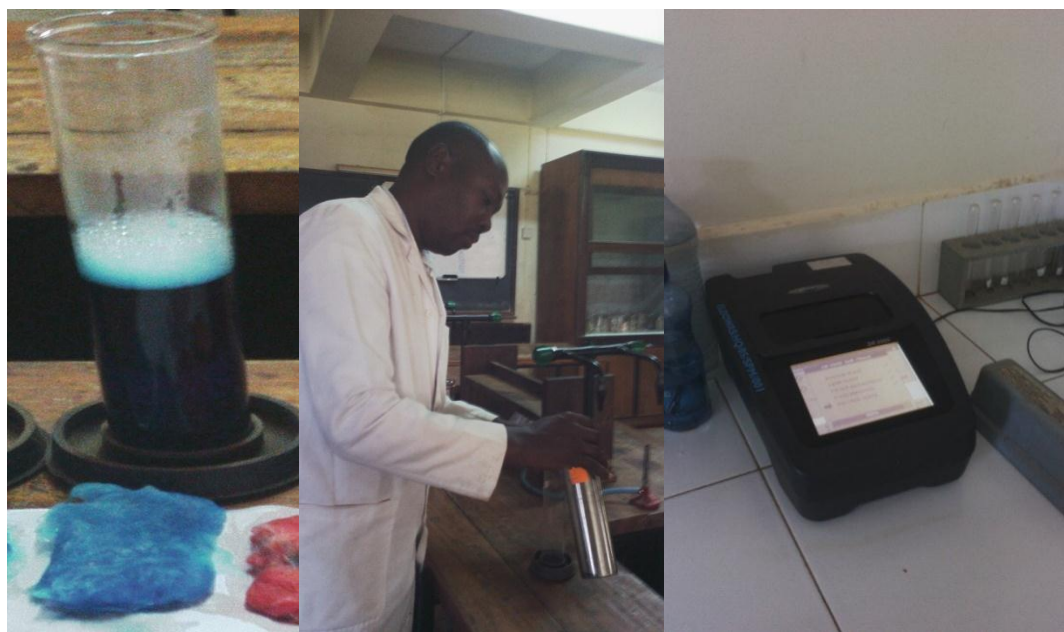
a) Methylene blue waste water after dyeing of acrylic fibre; b) Dyeing of acrylic fibre; c) UV Spectrophotometer for color determination`
