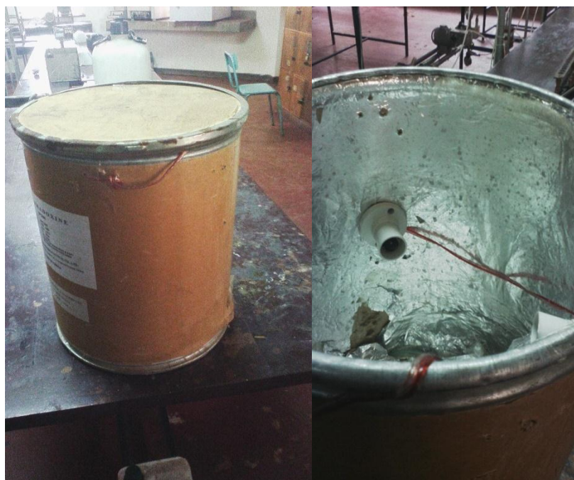
Figure B.6: Custom made photo-catalytic reactor.
