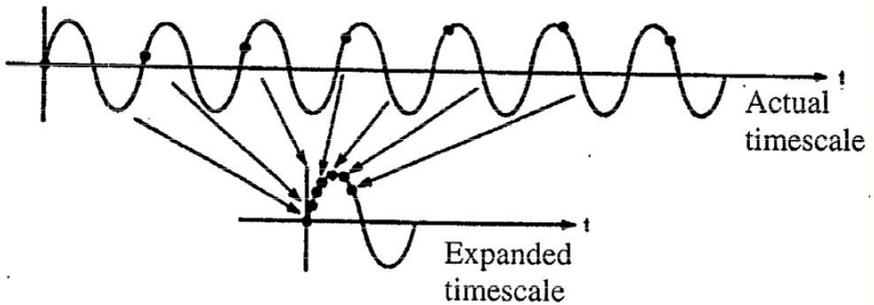
**Figure 3: The principle of sequential equivalent time sampling.  $\Delta T$  circuit**
