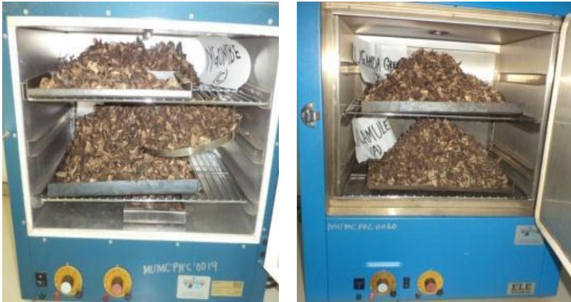
Plate 3.7: Oven drying of banana peels
